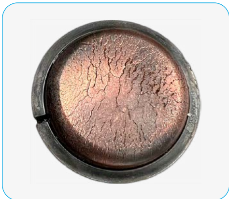
Thermal cracks at plunger
