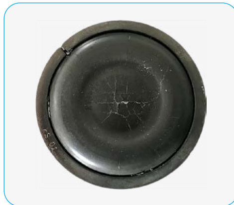
Crack line water leaks
